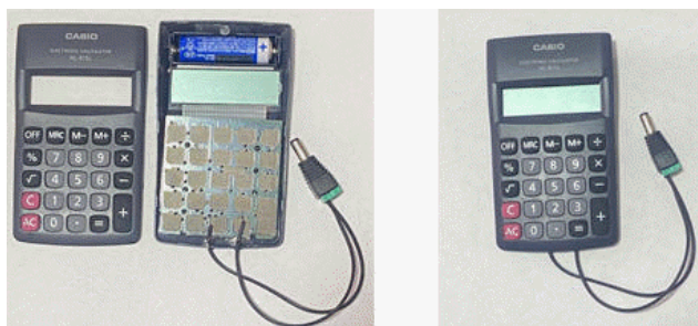
Figure 4. Connection points of the positive (“+”) and negative (“-“) poles of the CASIO HL-815L Calculator used to count inhalations
